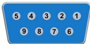
Figure 3-2 PDO-Profibus D-type connector pin out
